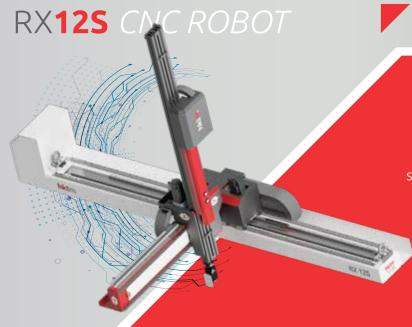
RX series robots, together with the knowledge of HKTM, sectoral experience and advanced technology, have been designed for plastic injection machines.
